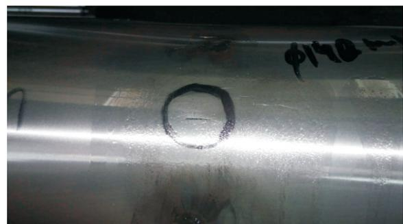
Any Magnetic particle build up having width more than 1.0mm and ratio of length to width more than three times will mean defect / crack.
