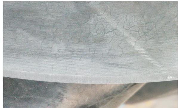
pressure. When applied on roll surface the softer areas will darken faster than the surroundings leaving a differential etch appearance. Cracks are also highlighted during an etching test. The reagent that enters the crack interface through capillary action. when the acid is cleaned the residual acid seeps out within the cracks and burns the area surrounding it. this test is also supplemented by UT testing on the located surface.
